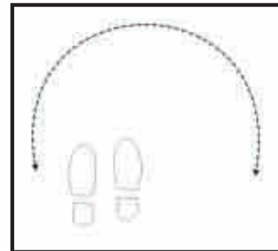
Figure 9. When the stem length is properly adjusted, the CZ-21 is balanced for sweeping a tight semicircle around the operator: wide to the right for right handers, wide to the left for left handers. Be sure to overlap your sweeps.
